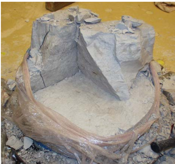
Figure 1. Photograph of the lower horizontal fracture plane in specimen 8 after test.
