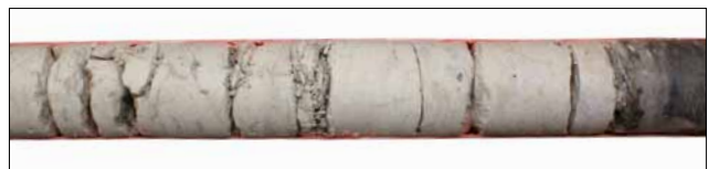
Limestone core sample taken with Geobor S- system
