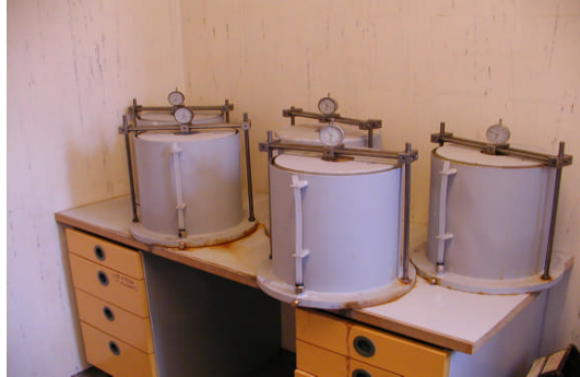
Photo No. 1. Five of the 12 test cylinders each with dial gauge on top and a saturation pipe outside the cylinder
